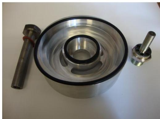
This adaptor is intended for the MkVII Jaguar which is fitted with a Tecalemit FA2678 filter head. This number should be found on a brass plate rivetted to the filter head; if you cannot find this number check with your supplier that this is the correct item for your car. It is not uncommon to find the filter head from one engine fitted to another so please check that you have the correct adaptor for your filter head. If in doubt contact your supplier.
